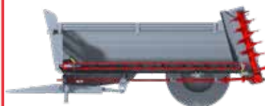
Drive line with transmission under the lowered axle (ideal for sloping terrain).
