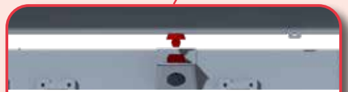
Noise-reducing silentblock for centering and lateral locking of the body on the chassis.
