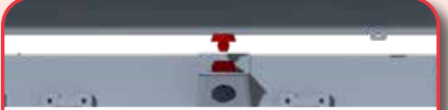
Noise-reducing silentblock for centering and lateral locking of the body on the chassis.
