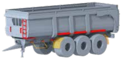
Folding aluminium ladder, galvanised side mudguards and pre-equipment for optional equipment (side bumper and thermoplastic mudguards).
