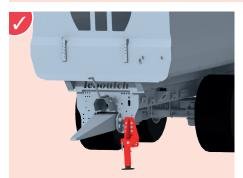
Hydraulic folding parking stand attached directly to the trailer chassis to free the drawbar and facilitate turning.
