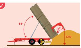
High-clearance rear door with hydraulic opening for easy unloading of silage with an extension and to avoid scraping the pile when tipping at the highest.
